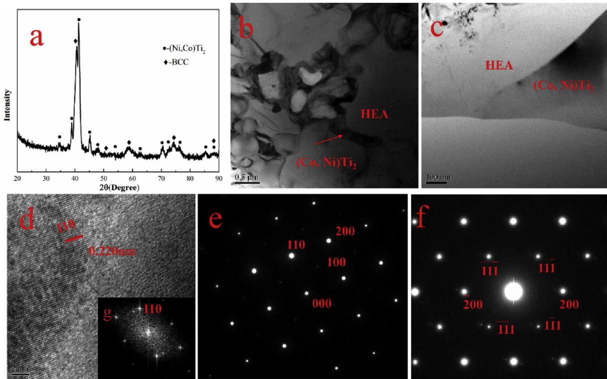
**Fig. 2.** XRD pattern of HEA coating (a); TEM images of complex HEA coating (b) and phase interface of BCC HEA/(Co, Ni)Ti<sub>2</sub> (c); HRTEM image of phase interface of BCC HEA/(Co, Ni)Ti<sub>2</sub> (d); SAED pattern of HEA phase (e) and (Co, Ni)Ti<sub>2</sub> phase (f); FFT image of HEA phase in Fig. 2d (g).
