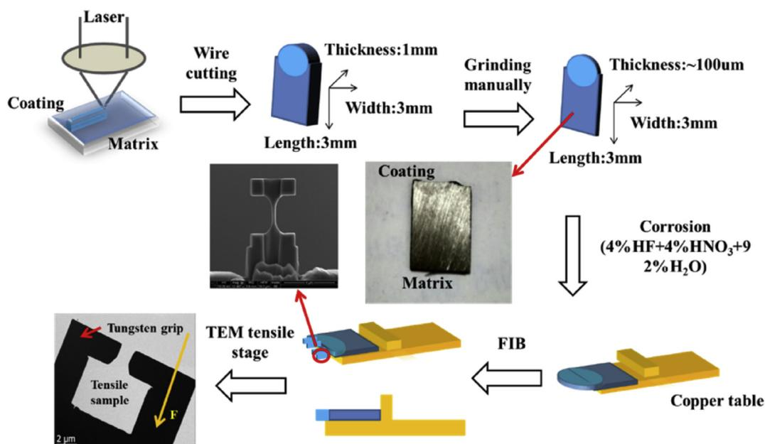
Fig. 1. Schematic diagram of tensile specimen preparation.
