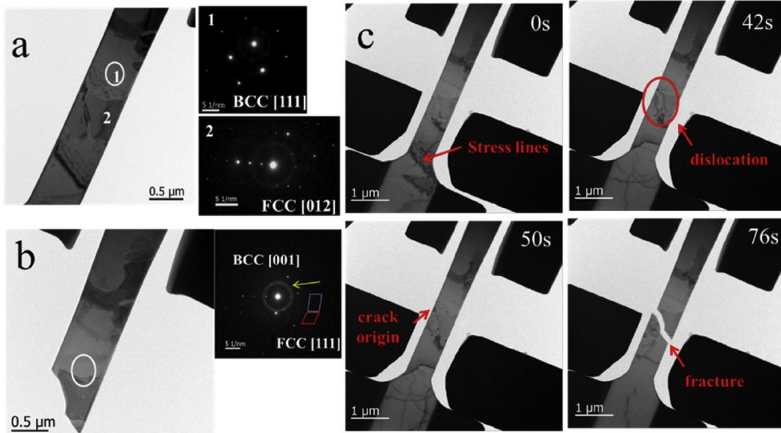
**Fig. 3.** (a) TEM images and corresponding SAED images before tensile testing; (b) TEM images and corresponding SAED images after tensile testing; (c) evolution of fracture process during *in situ* TEM tensile testing.
