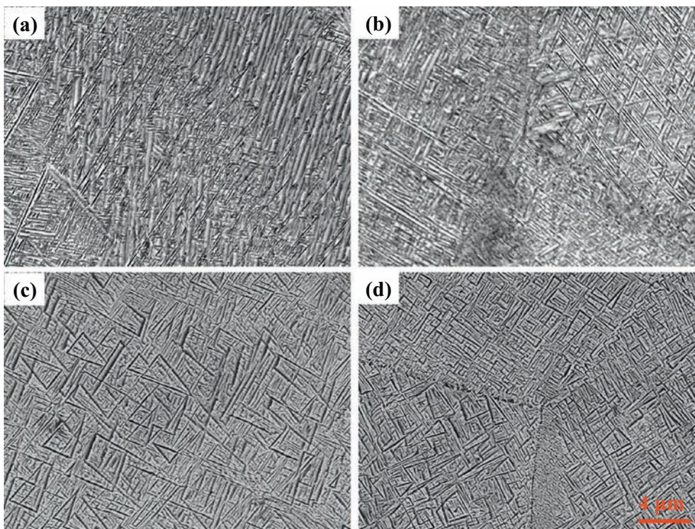
Fig. 3. SEM micrographs of the sample AC96-1: (a) intragranular  $\alpha$  precipitates and (b) grain boundary  $\alpha$  phase, and the AC96-2: (c) intragranular  $\alpha$  precipitates and (d) grain boundary  $\alpha$  phase.
