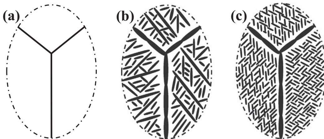
Fig. 9. Schematic illustration of the interface of grain boundary and intragranular microstructure under different heat treatment conditions: (a) Initial  $\beta$  grain boundary after the  $\beta$  solution treatment, (b) The single-step aged interface of grain boundary  $\alpha$  phase and intragranular precipitates, (c) The duplex aged interface of grain boundary  $\alpha$  phase and intragranular precipitates.
