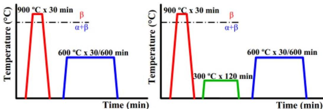
Fig. 1. Schematic illustration of different heat treatment approaches applied in this study.
