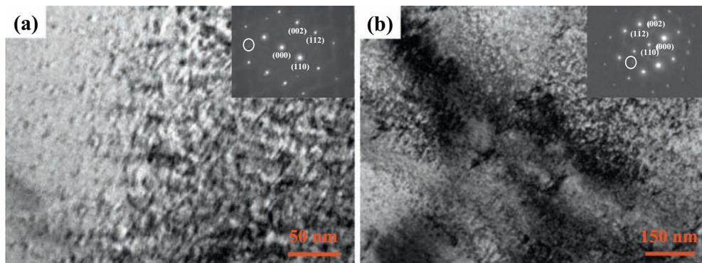
Fig. 8. Bright-field TEM images of Ti-55531 alloy after (a) the  $\beta$  solution treatment with air cooling and (b) the  $\beta$  solution treatment plus pre-ageing at 300 °C/120 min. Selected-area diffraction patterns were taken along the  $[110]_{\beta}$  zone axis.
