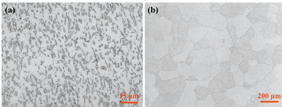
Fig. 2. Optical micrographs of Ti-55531 alloy under (a) as-received condition and (b)  $\beta$  solution-treated condition.
