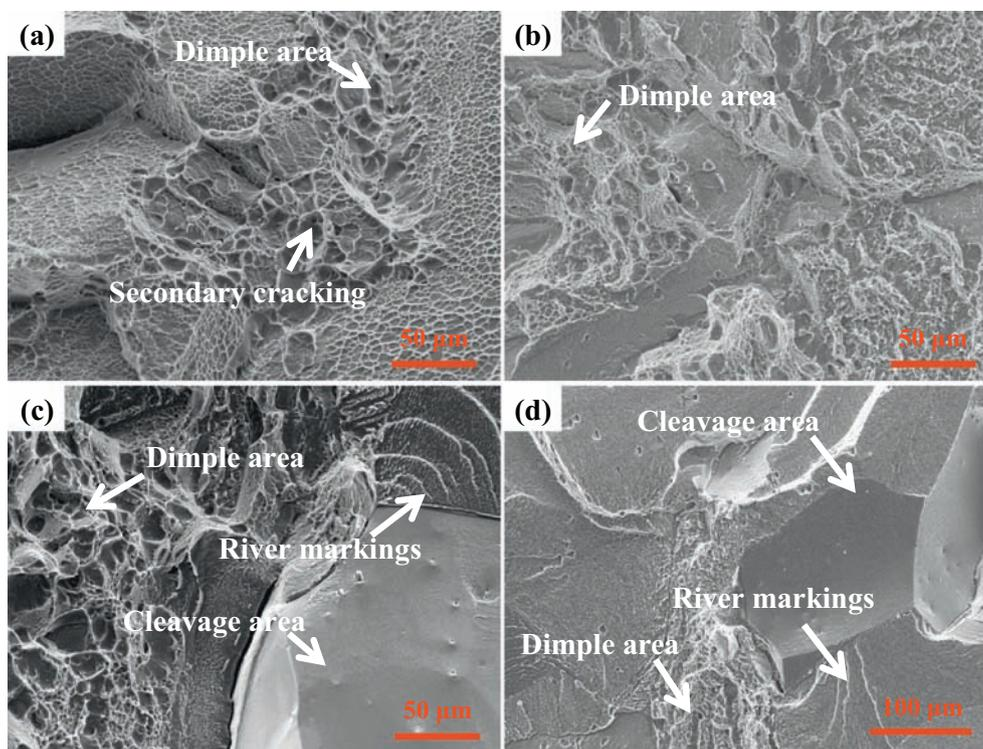
Fig. 6. SEM images of fracture surfaces of Ti-55531 alloy after  $\beta$  solution treatment plus various ageing ways: (a) AC96-1, (b) AC96-2, (c) AC936-1, (d) AC936-2.
