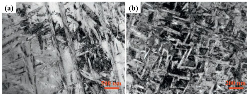
Fig. 7. High-magnification images of (a) AC96-1 and (b) AC936-1 showing intragranular acicular  $\alpha$  precipitates.
