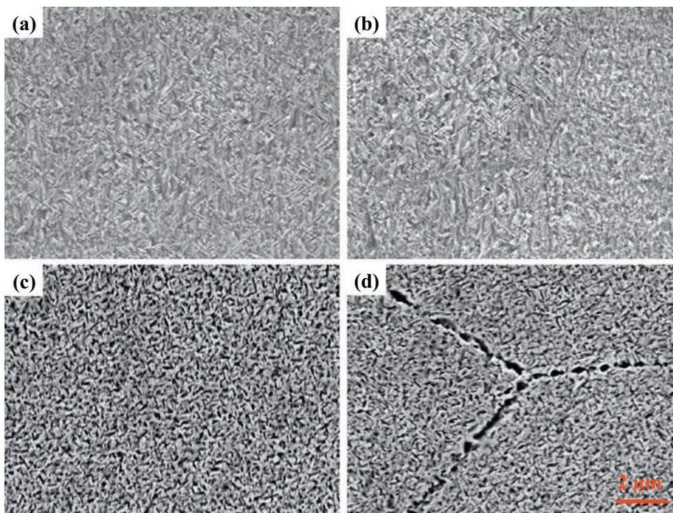
Fig. 4. SEM micrographs of the sample AC936-1: (a) intragranular  $\alpha$  precipitates and (b) grain boundary  $\alpha$  phase, and the AC936-2: (c) intragranular  $\alpha$  precipitates and (d) grain boundary  $\alpha$  phase.
