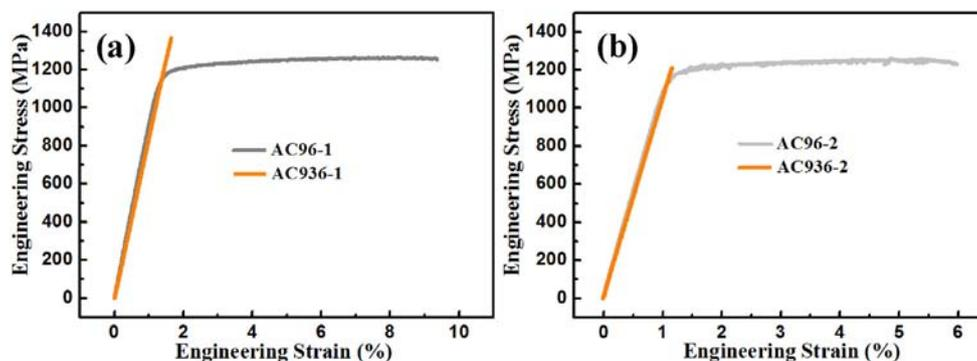
Fig. 5. Tensile engineering stress-strain curves of Ti-55531 alloy with various heat treatment conditions. The experiments were carried on at room temperature and strain rate of  $1.0 \times 10^{-4} \text{ s}^{-1}$ .
