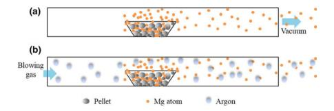
Fig. 2 Experimental setup of magnesium reduction under atmospheric pressure with flowing argon and the collected pure magnesium. a Experimental setup. b Condensed magnesium dendrites on the condenser. c Magnesium ingot made by melting the magnesium dendrites
